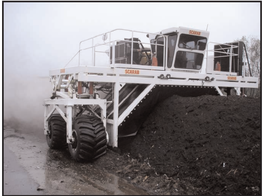
A Scarab machine turns the leaf windrows and it passes over. The steam is a result of the heat contained in the decaying leaf piles.
