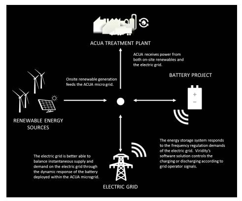
response to the signals in the grid. If there is excess supply, the batteries can charge up, and then switch to supply power back to the grid on a moment's notice.
